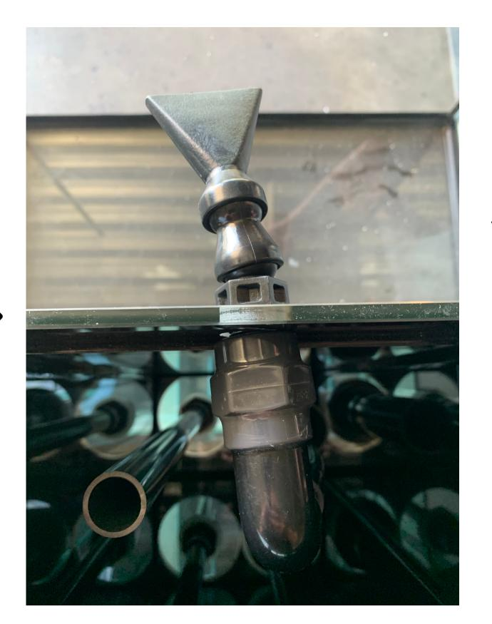
Fit the outlet pipe and screw the outlet in through the hole. **Note:** do not overtighten to prevent glass breakage
